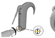
1. Turn the lock screw anticlockwise to unlock the tamperresistant battery cover (clockwise to lock).
